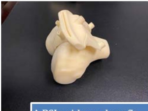
A PSI guide made to fit precisely over the end of the thighbone
